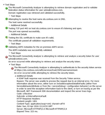
Figure 6-24: The results of the Office 365 Single Sign-On Test displaying an error connecting to the STS.
