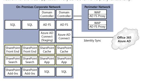
Figure 3-2: A SharePoint hybrid topology environment with redundancy.
