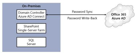
Figure 3-1: A simplified SharePoint hybrid topology environment with no redundancy
