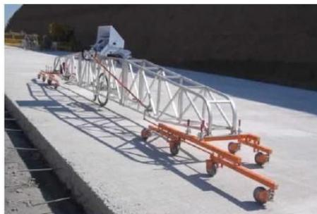
**Fig. 2.12. Perfilógrafo Rainhart**
