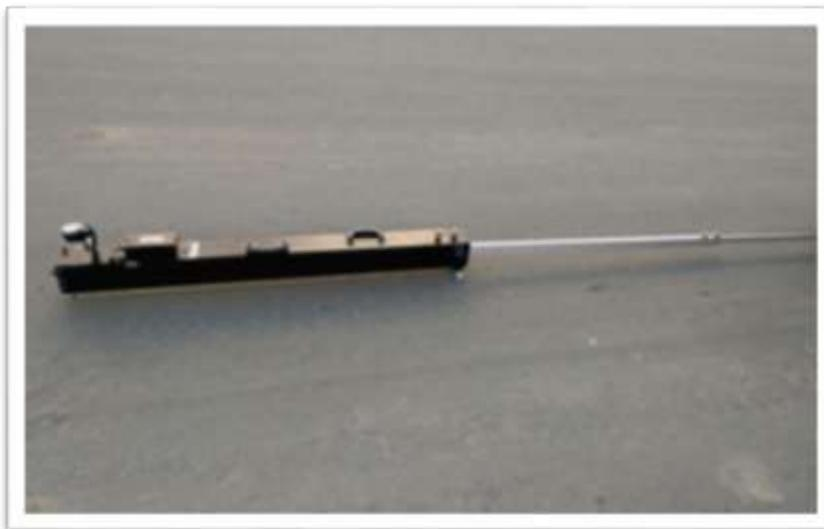
**FIGURA 3. 9: VIGA CON DIAL DIGITAL**
