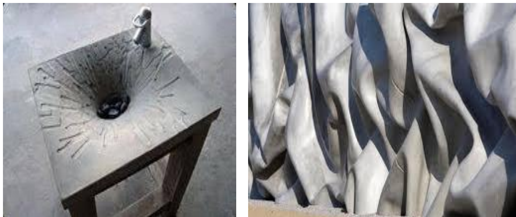
Figura N°21 Textura encofrado textil by Daniela y Crushedwall Walter Jack, Hormigón
