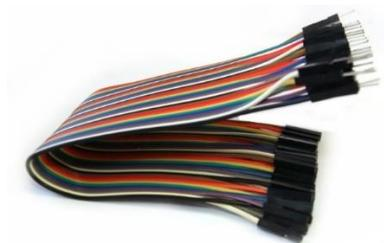
Figura 74: Cables jumper
