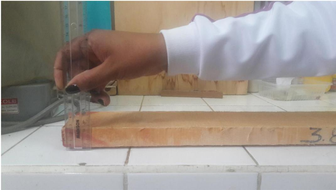
**Foto N° 17 Identificando defectos de torcedura**
