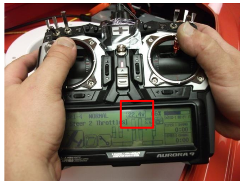
Battery voltage with motors at full power
