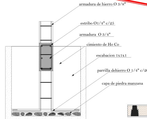
DETALLE DE ZAPATA Y COLUMNA
