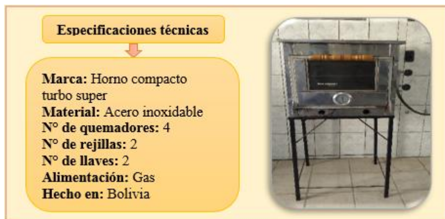
Figura 3.1. Horno semi-industrial a gas natural
