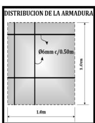
○ **PESO TOTAL DE HIERRO** =  $0.89 \text{Kg/m}^{2*} 1.1 = 0.98 \text{ kg/m}^{2}$
