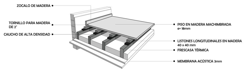
**DETALLE CONSTRUCTIVO PISO FLOTANTE - ESC. 1:10**
