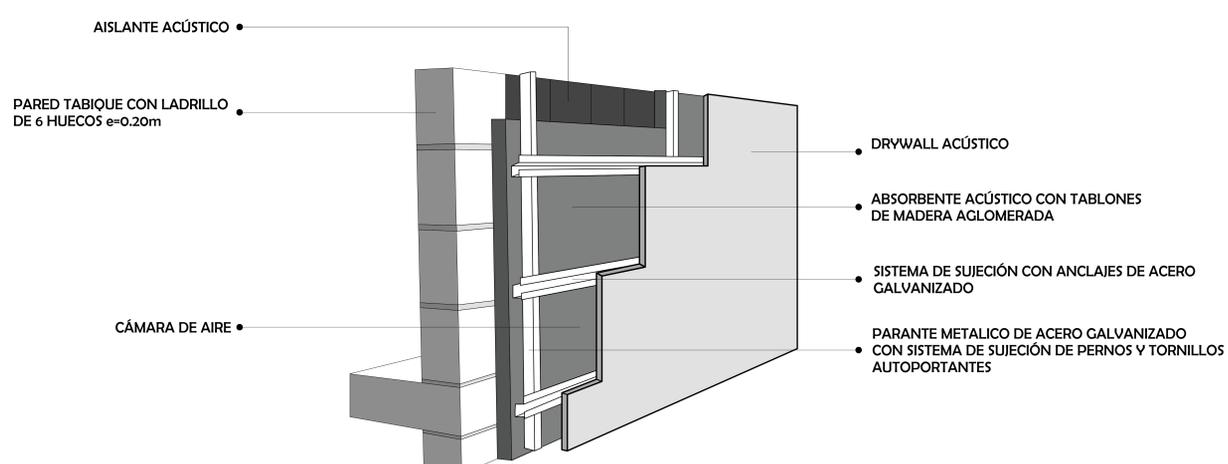
**DETALLE CONSTRUCTIVO MURO ACÚSTICO - ESC. 1:10**
