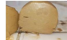
MEDIA ESPERA LATERAL DERECHA. – AGRIETAMIENTO POR CORTE CASI INEXISTENTES, CON TEXTURA SUAVE.
