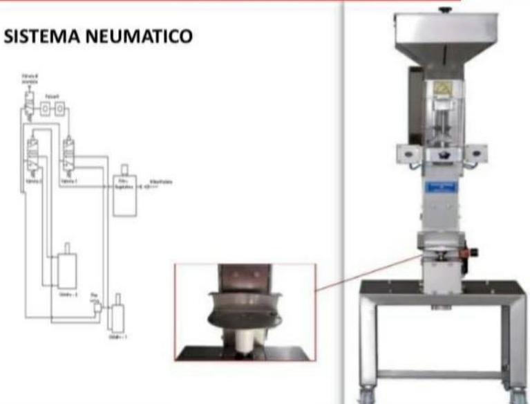
The diagram on the left illustrates the pneumatic system, showing a network of pipes, valves, and cylinders. A photograph in the center shows the physical machine, a tall stainless steel unit on a four-wheeled base. An inset image provides a close-up view of the corking mechanism, showing a cork being inserted into a wine bottle neck.
