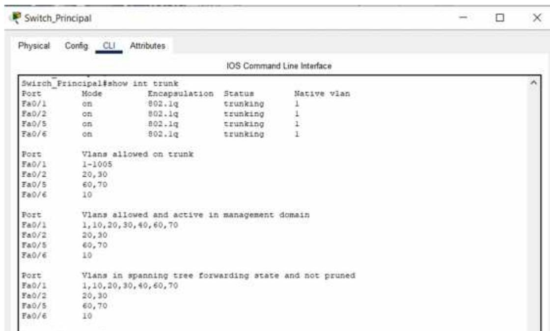
The screenshot shows a window titled "Switch\_Principal" with tabs for "Physical", "Config", "CLI", and "Attributes". The "CLI" tab is active, displaying the "IOS Command Line Interface". The command "Switch\_Principal#show int trunk" has been executed, resulting in the following output:
