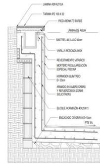
**DETALLE VASO FIGURA ESC: 1:10**
