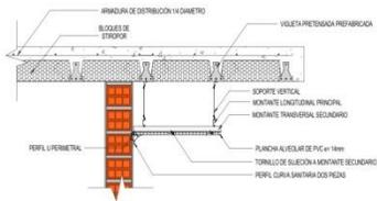
**FIGURA DE FALSO CIELO CON PVC ESC: 1:10**
