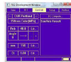
SonReb menu to evaluate the concrete strength combining the ultrasonic and concrete hammer measurements
