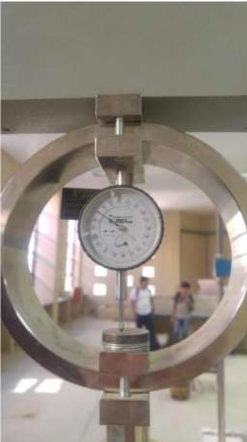
Fig.2.6 Anillo extensómetro cbr controls
