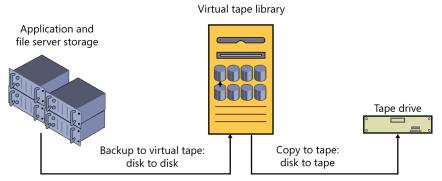
FIGURE 2-1 An illustration of the disk-to-disk-to-tape backup design.
