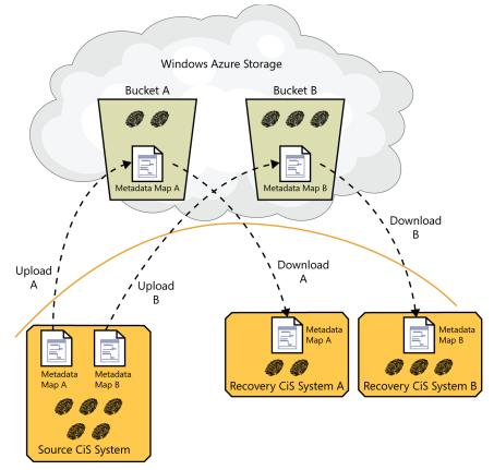
**FIGURE 3-4** The process of parallel recovery from data stored in two Windows Azure Storage buckets to two different recovery CiS systems.
