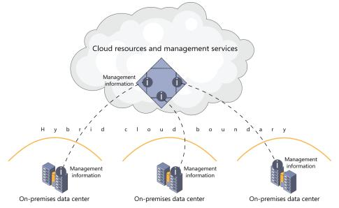
**FIGURE 1-1** Three on-premises data centers exchange management information with cloud resources and management services across the hybrid cloud boundary.
