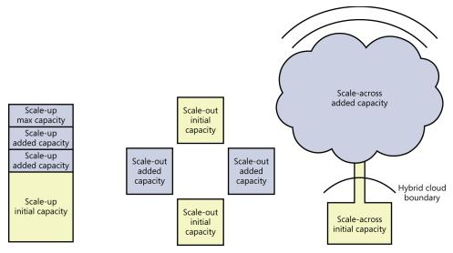
FIGURE 4-4 A comparison of storage scaling architectures.
