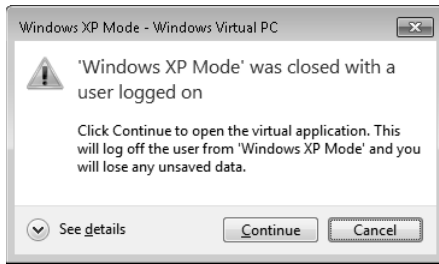
FIGURE 3-22 You must log off from the Windows XP Mode console window before the virtual application can start.
