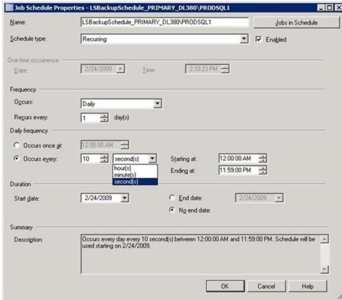
Figure 1: SQL Server 2008 Log Shipping user interface enables scheduling the jobs in hour, minute, or second frequency
