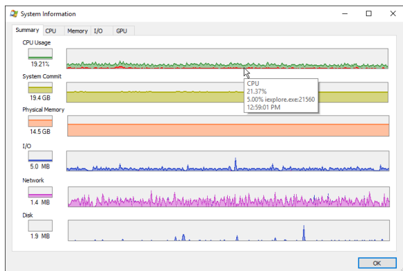
Figure 7-6: The System Information window shows real-time performance graphs for the current system,
