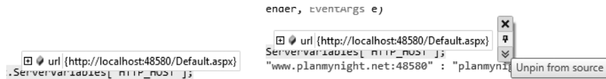
FIGURE 10-11 On the left is the pinned DataTip, and on the right is the DataTip management bar
