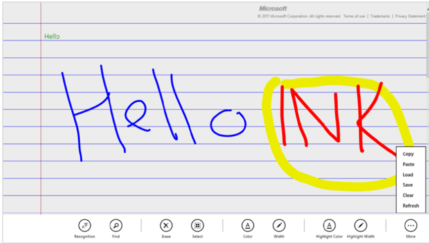
FIGURE 9-9 The Input Ink sample with many commands on its app bar. The green “Hello” text in the upper left was generated by selecting the Hello ink and tapping the Recognition command.
