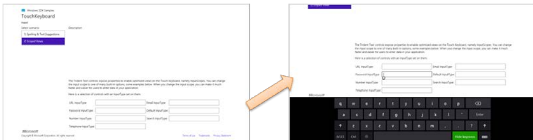
FIGURE 9-6 When the soft keyboard appears, Windows will automatically slide the app page up to make sure the input field isn't obscured.
