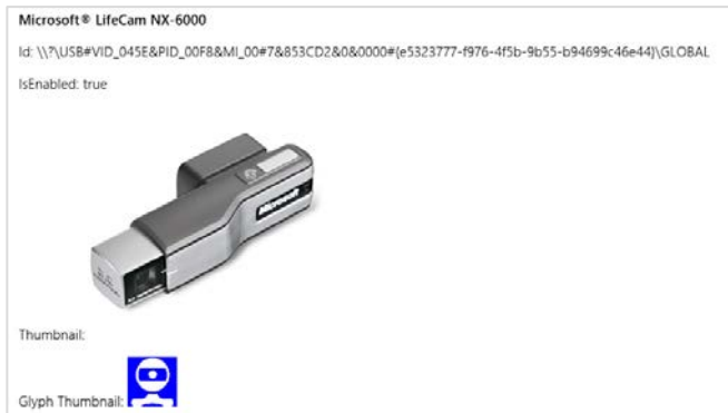
FIGURE 15-3 Sample device enumeration output for a webcam—which perfectly represents the one attached to my monitor.
