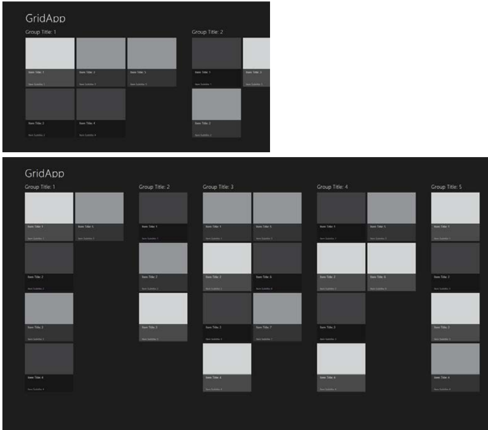
FIGURE 6-7 Adaptive layout in the Grid App project template shown for a 1366x768 display (top) and a 2560x1440 display (bottom).
