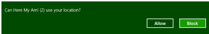
FIGURE 2-18 A typical consent popup, reflecting the user's color scheme, that appears when an app first tries to call a brokered API (geolocation in this case). If the user blocks access, the API will fail, but the user can later change consent in the Settings/Permissions panel.
