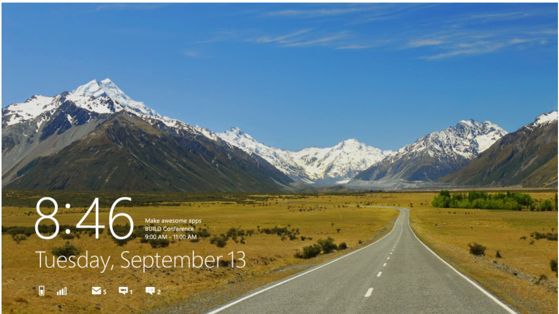
FIGURE 13-9 A typical lock screen. Up to seven apps can display badges along the bottom of the screen; one app can display text next to the clock.
