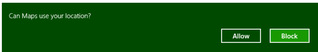
FIGURE 1-7 A typical user consent dialog that's automatically shown when an app first attempts to use a brokered capability. This will happen only once within an app, but the user can control their choice through the Settings charm's Permissions command for that app.
