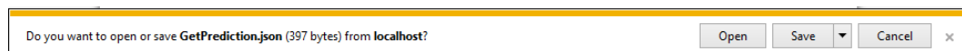
FIGURE 4-43 A JSON file is returned to the browser after a web request to the ASP.NET Web API web service with the income prediction results.
