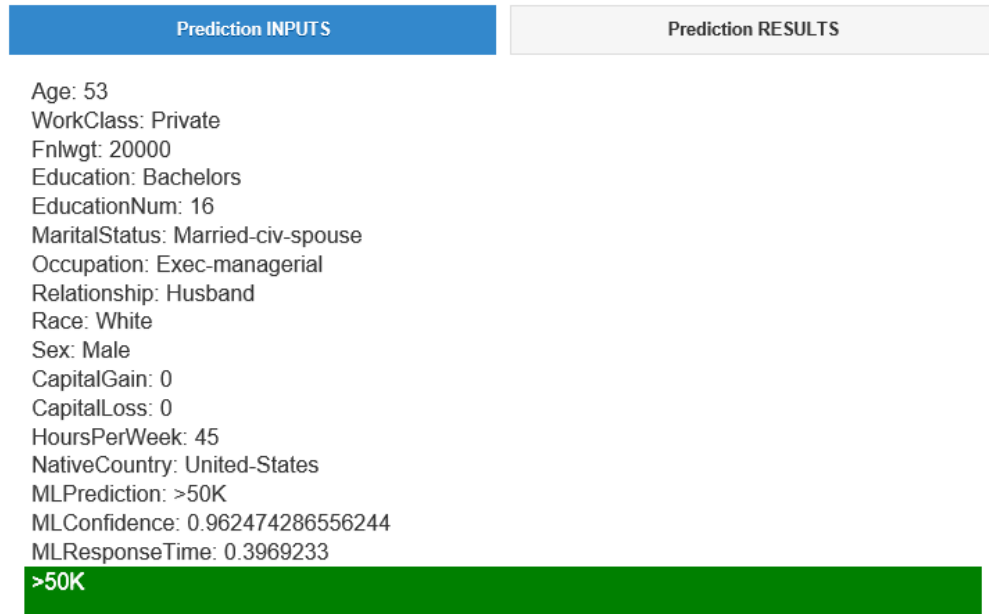
FIGURE 4-45 The results of a call to our new ASP.NET Web API web service displayed in a jQuery Mobile web application.
