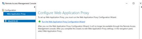
Figure 6-11: You can start the Web Application Proxy Configuration Wizard via the Remote Access Management Console.
