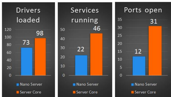
Figure 6-2: Default functionality comparison between Nano Server and Server Core
